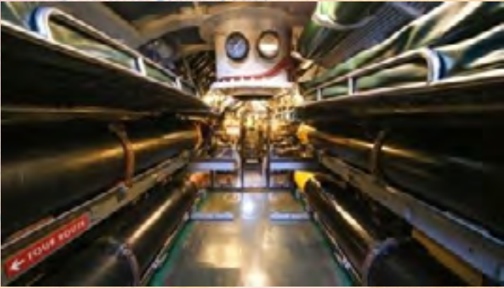
Sleeping racks above unarmed torpedoes. (WWII submarine, USS Pampanito (SS 383) memorial submarine. San Francisco.)
